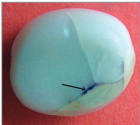
Figure 1. Dye penetration between original veneer and repair material (see arrow).
