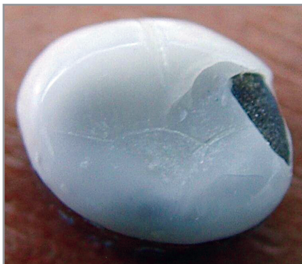
Figure 2. Extents of fractures varied among Class II and loss of one third of the original veneer material (original magnification X10).
