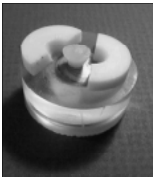
Fig 1. Jig and composite resin cone on embedded tooth specimen
