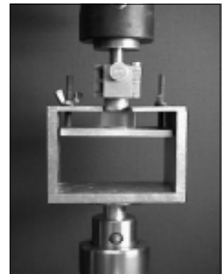
Fig 3. Specimen attached to Instron machine with a self-aligning system for tensile bond strength test
