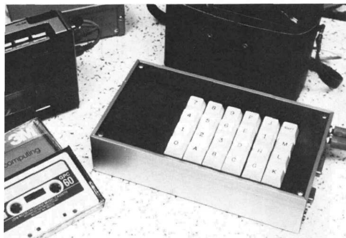
Figure 2. Microprocessor Operated Recording Equipment (MORE).
