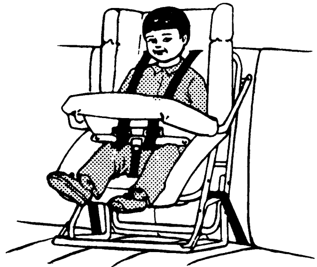
FIG 4. A convertible seat with a shield: the upper diagram shows the infant position, while the lower diagram shows the toddler position.
