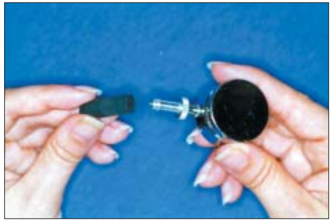
Fig 3. Step 2: Insert Luer adapter into one end of rubber tubing.
