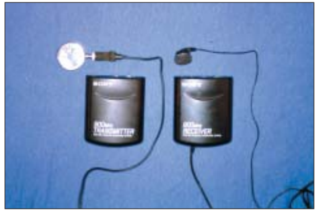
Fig 5. Completed stethoscope transmitter and receiver.
