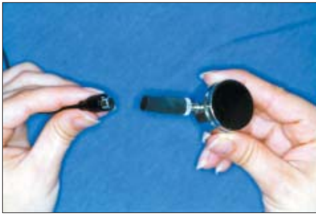
Fig 4. Step 3: Insert transmitter microphone into other end of rubber tubing.
