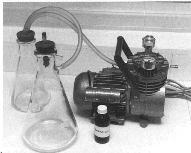
Fig 2. The vacuum suction apparatus for dye penetration of root canals.
