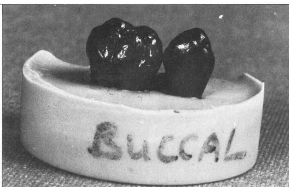
Figure 1a. A molar and premolar tooth painted with an acid resistant varnish and set up in interproximal contact in a silicone block at commencement of the study. Window regions of enamel have been left exposed on the mesial and distal proximal surfaces for the creation of artificial caries-like lesions.
