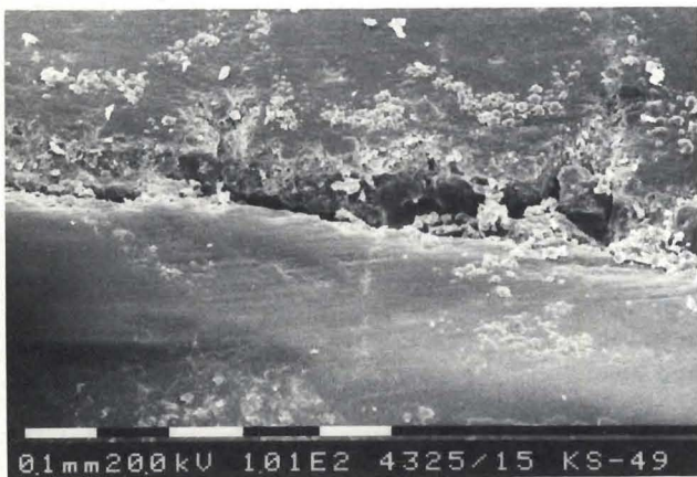
Figure 7. SEM micrograph of adaptation of Ketac Silver to the gingival floor, showing different gap widths along the margin. Top: Ketac Silver; Bottom: enamel.
