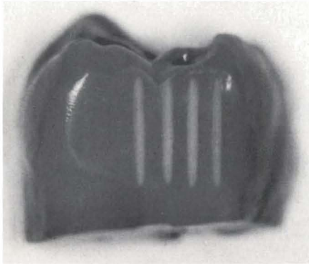
Figure 1. A photograph of the specimen with 4 grooves and coated with nail varnish before exposure to the demineralized solution.
