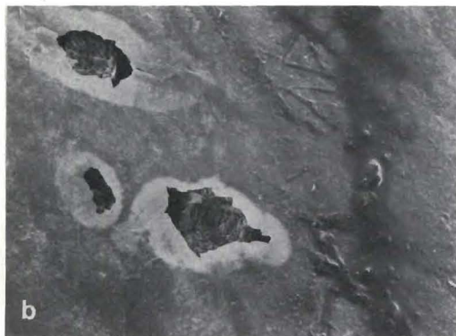
Figure 2b. Detail of Figure 2a showing the etched area with undermining of the reaction products on the enamel. (Mag. x 300 x 0.54).
