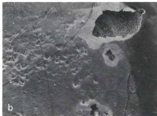
Figure 3b. Detail of Figure 3a showing the etched area with undermining of the reaction products on the enamel. (Mag. x 300 x 0.54).
