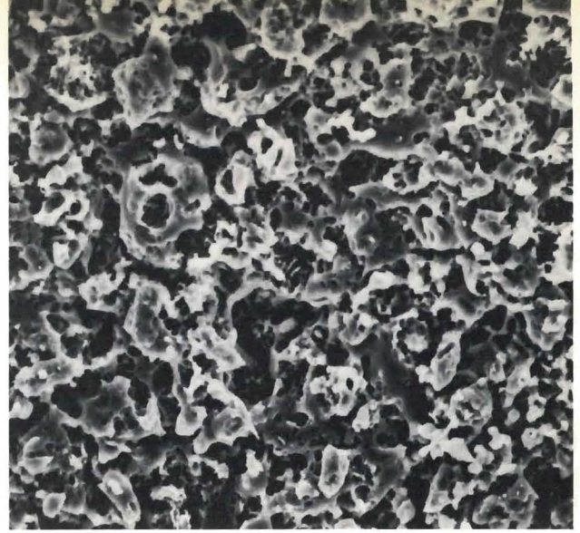
Figure 5. SEM photograph of an etched porcelain surface fired against the porcelain inlay investment. Surface was etched for 1.5 minutes. Magnification is 500x.
