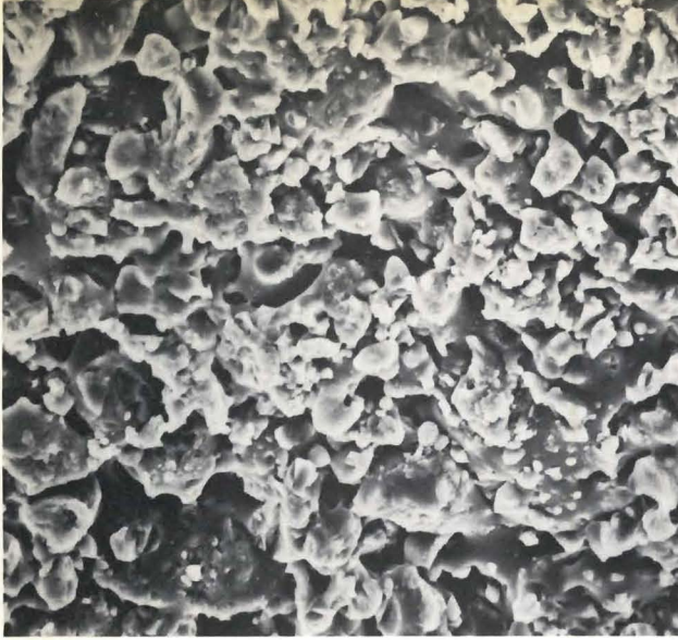
Figure 4. SEM photograph of an unetched porcelain surface fired against the porcelain inlay investment. Magnification is 500x.
