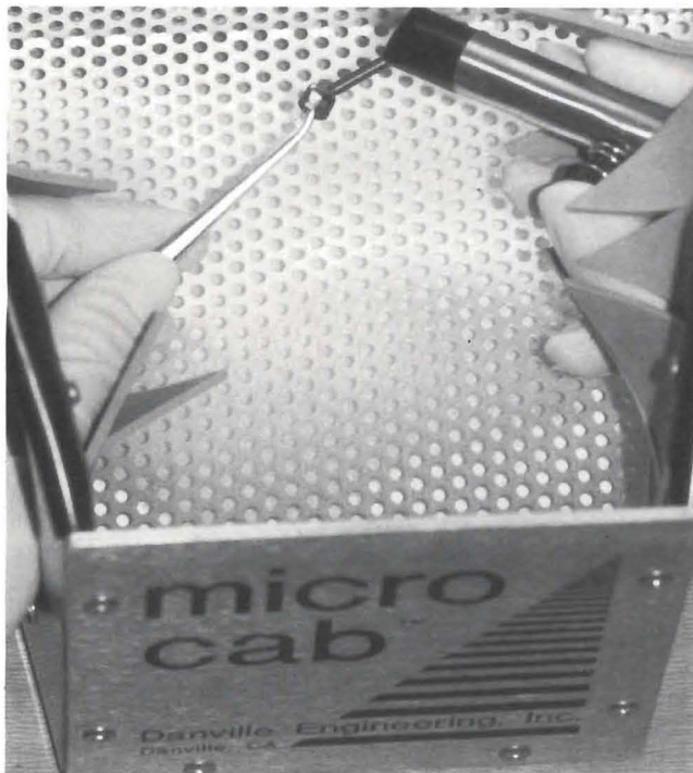
Figure 1. Fitted stainless steel crowns are sandblasted with aluminum oxide for two to four seconds.
